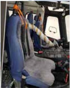
Intercept packaging reduces the overall cost of maintaining an out-of-service helicopter or for protection during shipping and transport. Intercept Technology™ completely controls and neutralises the environment of corrosive elements such as chlorides and sulphides around and within the aircraft.
